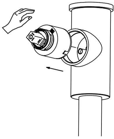
**SOSTITUZIONE AERATORE / AERATOR REPLACEMENT**
